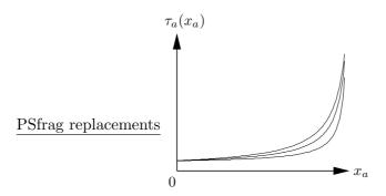
FIGURE 1. Typical link delay functions. Here,  $x_a$  is the flow on arc a, and  $\tau_a(x_a)$  is the associated travel time.
