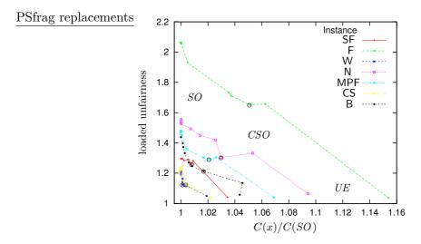
FIGURE 15. Tradeoff between efficiency and unfairness. For all instances, we plot the tradeoff curve between the efficiency (the cost of the solution over the cost of the system optimum) vs. the loaded unfairness. The left area of the graph corresponds to system optima (SO), the lower area corresponds to user equilibria (UE), and the circled data-points (denoted with 'o') correspond to constrained system optima with  $\varphi = 1.02$  ( $CSO^{1.02}$ ).
