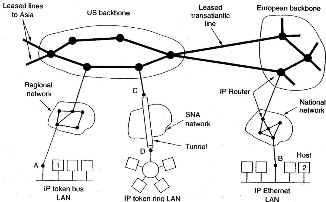
Figure 1: High-level structure of the Internet, showing LANs, gateways, regional networks and backbones.
