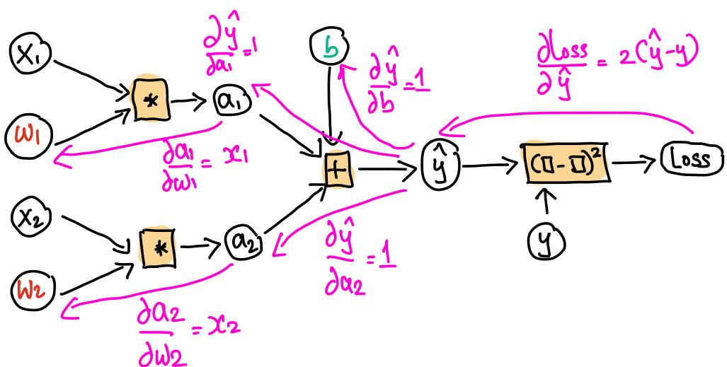
To calculate  $\frac{\partial \text{Loss}}{\partial \text{any parameter}}$ , start from the loss and travel backwards to the parameter, multiplying the partial derivatives as you go.
