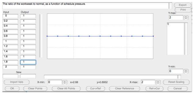
The input, schedule pressure, runs from 0 to 2 in steps of 0.2. The output, for the base case, is constant at 1.0 (no over- or undertime). You can try different policies for workweek by changing the values of the relationship in the simulation dialog box when you run the model.
