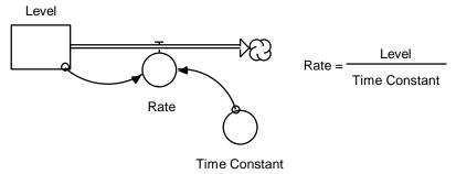
The Rate is equal to the Level divided by the Time Constant, or to the Level multiplied by the reciprocal of the Time Constant (the fraction 1/Time Constant).
