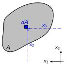
First moment of area Given an area A of any shape in the  $x_2$ - $x_3$  plane (as is the case for the cross section of a beam), the first moments of area with respect to the two axes are given respectively by:
