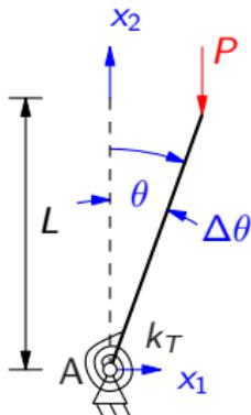
$$\begin{aligned}\sum M^{(A)} = 0 : & \Rightarrow -P \sin(\Delta\theta)L + k_T \Delta\theta = - \underbrace{I_A}_{>0} \ddot{\theta} \\ & \Rightarrow -I_A \ddot{\theta} = (k_T - PL) \Delta\theta\end{aligned}$$
