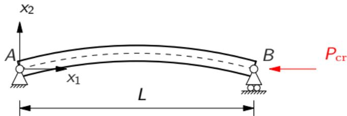
Note: Higher critical loads and their associated mode shapes can be reached if the column is "artificially restrained" at lower bifurcation loads.
