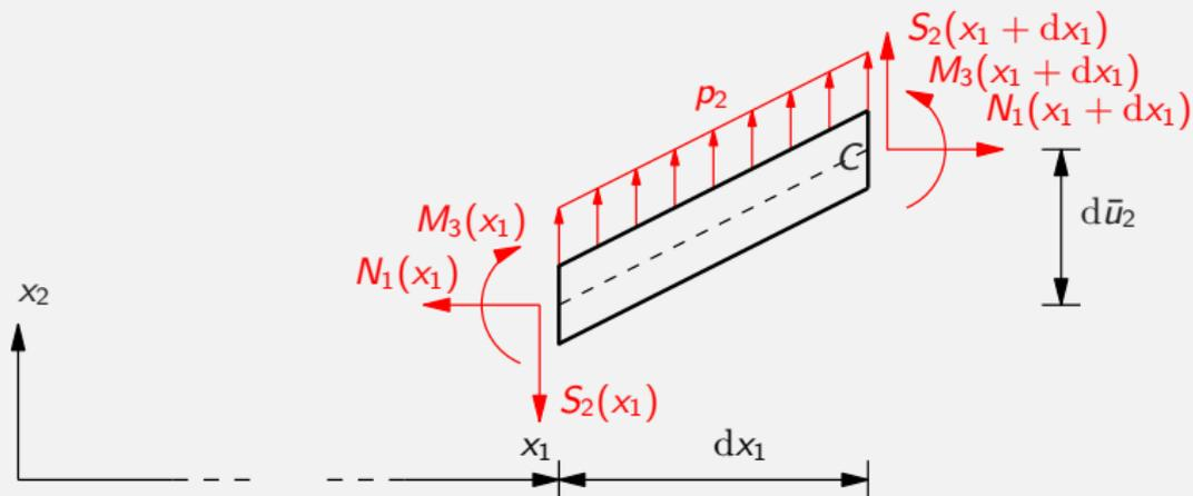
$$\begin{aligned}\sum M_3^{(C)} = 0 : & M_3(x_1 + dx_1) - M_3(x_1) + dx_1 S_2(x_1) \\ & - d\bar{u}_2 N_1(x_1) = 0 \\ \Rightarrow & \frac{dM_3}{dx_1} + S_2 - N_1 \frac{d\bar{u}_2}{dx_1} = 0\end{aligned}$$
