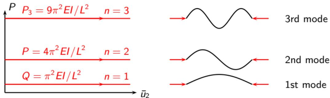
The lowest buckling load (obtained for  $n = 1$ ) is the one for which buckling occurs:
