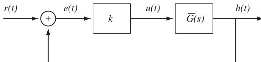
That is, the control input  $u(t)$  (normalized throttle) is a gain  $k$  times the error,  $e(t)$ , which is the difference between the altitude  $h(t)$  and the altitude reference  $r(t)$ . The transfer function from  $r(t)$  to  $h(t)$  can be shown to be
