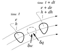
Over the short time interval dt, the CV undergoes a *process* where it receives work  $\delta w$  and heat  $\delta q$  from its surroundings, both per unit mass. This process results in changes in the state of the CV, described by the increments de, dh, dp... The first law of thermodynamics for the process is
