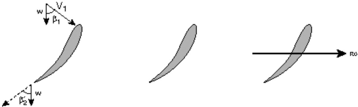
a) Draw velocity triangles in the relative and absolute frames for the different blade speeds shown below for both the inlet and exit to the rotor. (Note the inlet velocity components form a 3-4-5 triangle.)
