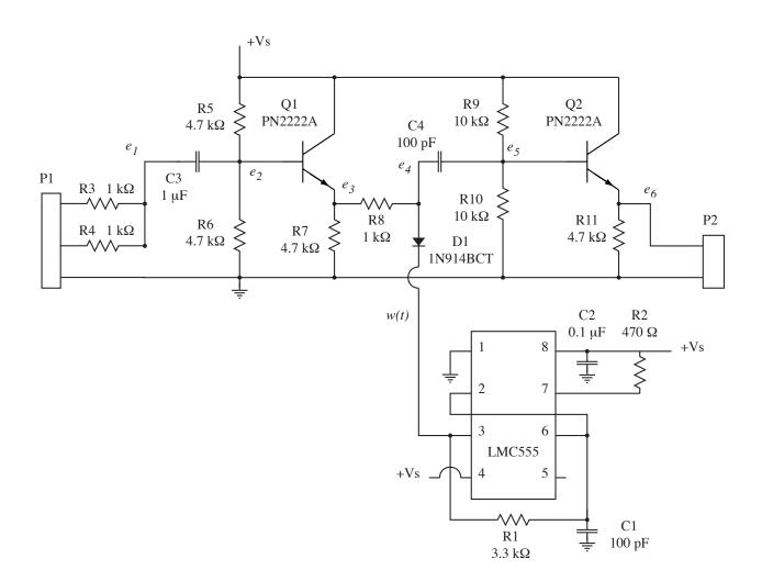
Figure 2: Amplitude Modulation Circuit
