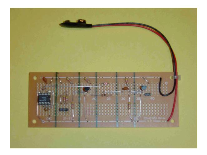
Figure 3: Assembled Amplitude Modulation Circuit.
