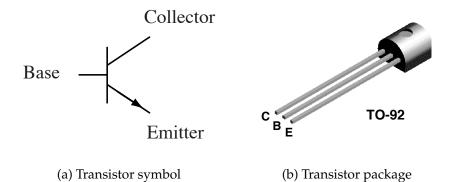
Figure 4: PN2222A Transistor.
