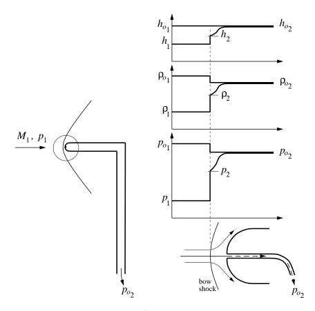
In addition, we also have  $M_2$  and  $p_2/p_1$  as functions of  $M_1$  from the earlier normal-shock analysis. Combining these produces the relation between the  $p_{o_2}$  measured by the pitot probe, the static  $p_1$ , and the required flow Mach number  $M_1$ . After some manipulation, the result is the *Rayleigh Pitot tube formula*
