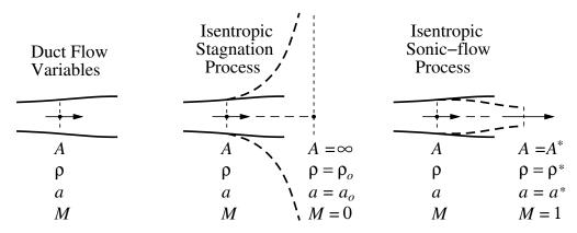
The resulting quantities at the hypothetical sonic throat are denoted by a ()\* superscript. The advantage of the sonic-flow process is that it produces a well-defined *sonic throat area*
