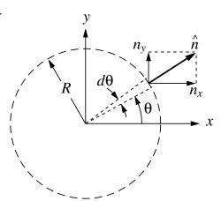
Breaking up the resultant force/span (2) into separate x- and y-components, and dividing by  $\frac{1}{2}\rho V_{\infty}^2 2R$ , we obtain expressions for the drag and lift coefficients.
