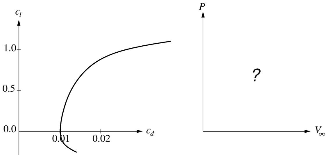
b) Determine the form of the  $P(V_\infty)$  relation in level flight, and plot it for the range  $c_\ell = 0.1 \dots 1.2$ . Any constant multiplicative factors on the  $P$  and  $V_\infty$  axes are not important – only the shape of the curve is of interest. Hint: Simplest approach is to plot  $P(c_\ell)$  versus  $V(c_\ell)$  with  $c_\ell$  as a dummy parameter.
