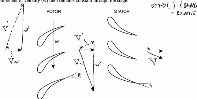
a) Draw the velocity triangles. Is this a compressor or a turbine?
