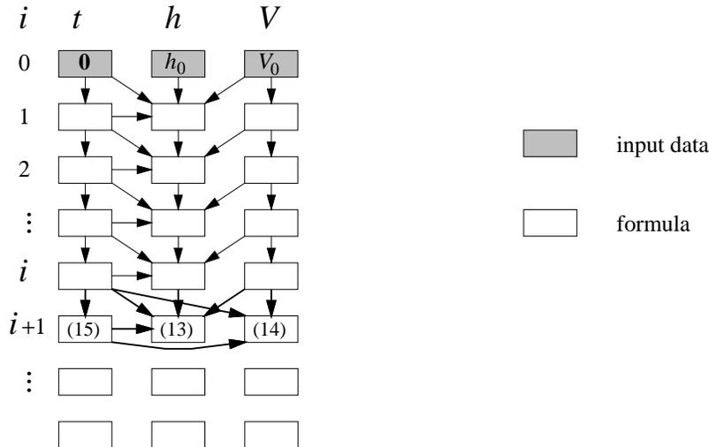
Figure 4: Spreadsheet for time stepping. Arrows show functional dependencies.
