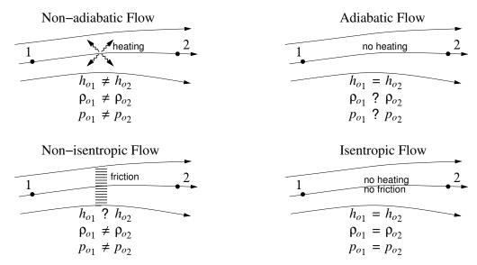
For the adiabatic case, a unique total enthalpy  $h_o$  can be assigned to the whole streamline. Then for any point on the streamline we have
