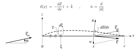
To force the total velocity to be parallel to the camberline, we now apply the flow tangency condition  $\vec{V} \cdot \hat{n} = 0$ . Performing the dot product and removing the unnecessary factor  $1/|\vec{n}|$  gives the fundamental equation of thin airfoil theory.
