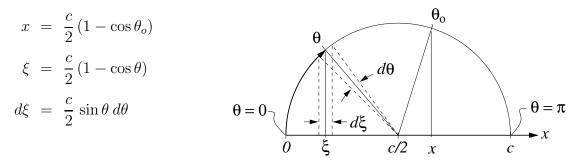
As shown in the figure,  $\theta$  runs from 0 at the leading edge, to  $\pi$  at the trailing edge. Since x and  $\theta$  are interchangable, functions of x can now be treated as functions of  $\theta$ . Equation (1) then becomes
