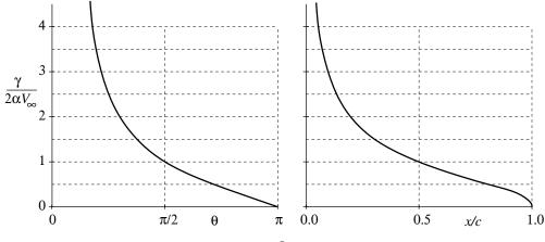
Note that at the trailing edge,  $\gamma = 0$  as required by the Kutta condition, and that at the leading edge  $\gamma \to \infty$ . The latter is of course not physical, although the singularity is weak (integrable), and the integrated results for  $c_{\ell}$  and  $c_m$  are in fact valid.
