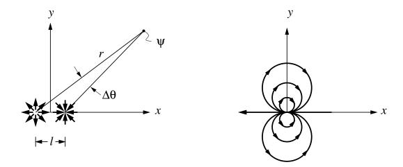
A similar limiting process can be used to produce the doublet's potential function.
