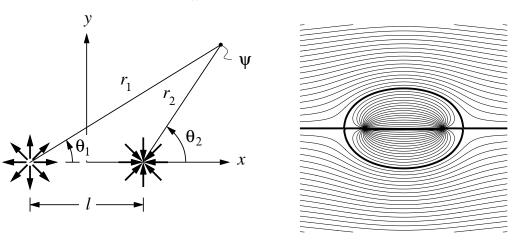
The figure on the right shows the streamlines of the combined flow. The heavy line again indicates the dividing streamline, which traces out a *Rankine oval*. All the streamlines inside the oval originate at the source on the left, and flow into the sink on the left. The net volume outflow from the oval is zero. Again, the dividing streamline could be replaced by a solid oval body of the same shape. The flow outside the oval then corresponds to the flow about this body.
