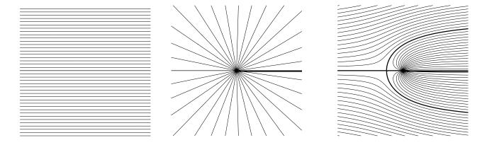
The bullet-shaped heavy line on the combined flow corresponds to the *dividing streamline*, which separates the fluid coming from the freestream and the fluid coming from the source. If we replace the deviding streamline by a solid semi-infinite body of the same shape, the flow about this body will be the same as the flow outside the dividing streamline in the superimposed flow.
