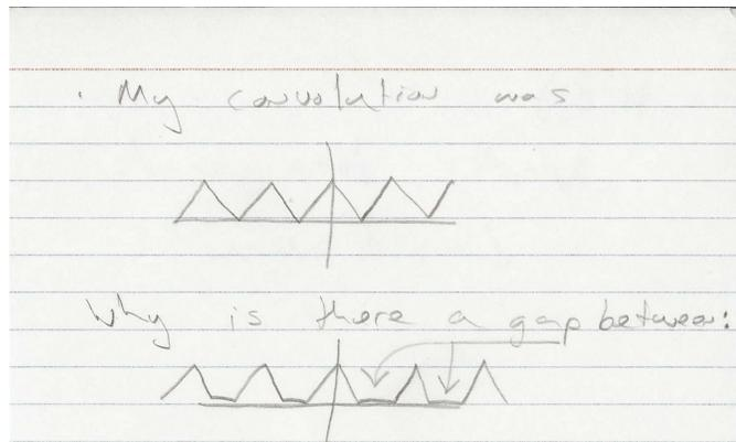
The width of each triangle is (twice) the bandwidth of the sampled signal. The distance between the peaks of adjacent triangles is the sampling frequency. If the sampling frequency is greater than twice the the bandwidth, then there is a gap between triangles. This is the whole point — we want there to be same gap.
