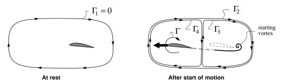
the airfoil must be zero as well. When the airfoil is set into motion, it will develop a nonzero circulation,  $\Gamma_4$  in the figure. Experimental flow observations show that a *starting vortex* of circulation  $\Gamma_3$  is shed from the trailing edge. This shedding is associated with the Kutta condition being satisfied for every instant in time. The vortex is swept downstream as seen by an observer on the airfoil.
