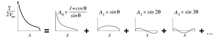
already been determined, and are now merely used to construct  $\gamma(\theta)$  by simple summation of the series. This  $\gamma(\theta)$  will now be integrated to obtain the lift force and moment.
