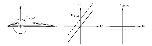
These results are subject to the assumptions inherent in thin airfoil theory. In practice, they are surprisingly accurate even for relatively thick or highly-cambered airfoils. It appears to be better at predicting trends (with camber,  $\alpha$ , etc) than absolute numbers. When used merely as a conceptual framework for understanding airfoil behavior rather than for quantitative predictions, thin airfoil theory is highly applicable to almost any airfoil.
