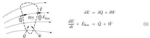
where the second rate form is obtained by dividing by the process time interval dt, and including the contribution of flow in and out of the volume.
