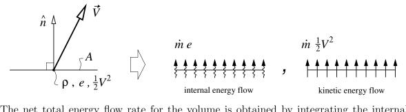
The net total energy flow rate for the volume is obtained by integrating the internal and kinetic energy flows over its entire surface.
