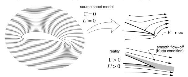
On real airfoils the flow always flows smoothly off the sharp trailing edge, with no large local velocities. This smooth flow-off is known as the *Kutta condition*, and it must be faithfully duplicated in any flow model which seeks to predict the lift correctly. Changing the streamline pattern to force the flow smoothly off the trailing edge requires the addition of circulation, which implies that vortices must be included in the flow representation in some manner.
