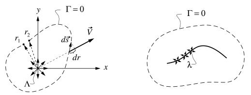
This zero-circulation property of source sheets has severe consequences for flow representation. Any aerodynamic model consisting only of a freestream and superimposed source sheets will have  $\Gamma = 0$ , and hence L' = 0 as well. Hence, lifting flows cannot be represented by source sheets alone.
