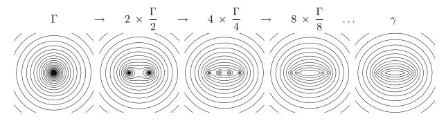
Like with the source sheet strength  $\lambda$ , the units of  $\gamma$  are length/time (or velocity).
