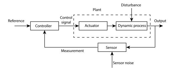
Typically, we are interested in cases where the plant and controller are linear and timeinvariant, or can be modeled as such. Then we can represent components as transfer functions:
