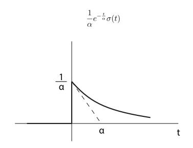
So, net effect is that addition of the pole will smooth the original step response, increasing the rise time, and reducing the overshoot,
