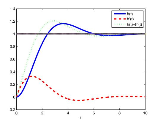
So a zero (with  $\alpha>0)$  tends to speed up time response increase overshoot. Note that the zero is at root of
