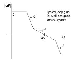
In this case, the phase at cross-over will be a weighted average of  $-90^{\circ}$  (weighted a lot),  $-180^{\circ}$  (weighted some), and  $0^{\circ}$  (weighted hardly at all). So the phase will be between  $-90^{\circ}$  and  $-180^{\circ}$ , with probably reasonable PM.
