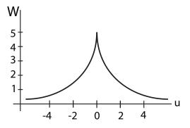
Note that 92% of area of W(u) is within  $\pm 1$  decade of the center. So the phase is nearly completely determined by the slope of M within ~1 decade.
