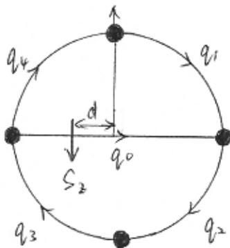
$d$  = horizontal distance between shear center and centroid.
