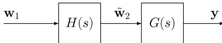
– Then must design filter  $H(s)$  so that the output is a noise  $\tilde{w}_2$  that has the frequency content that we need
