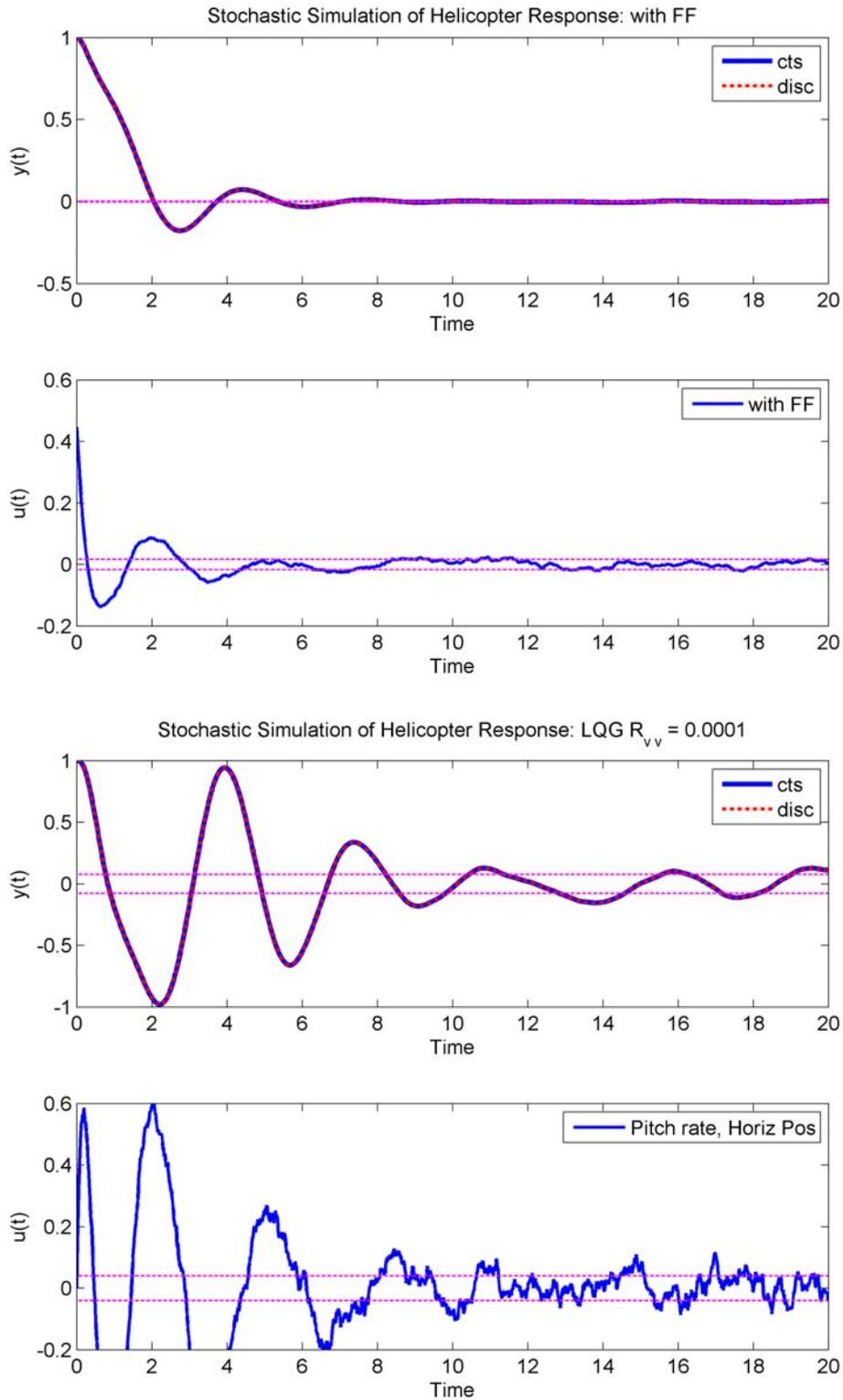
Figure 12.5: Second LQR with disturbance feedforward compared to LQG
