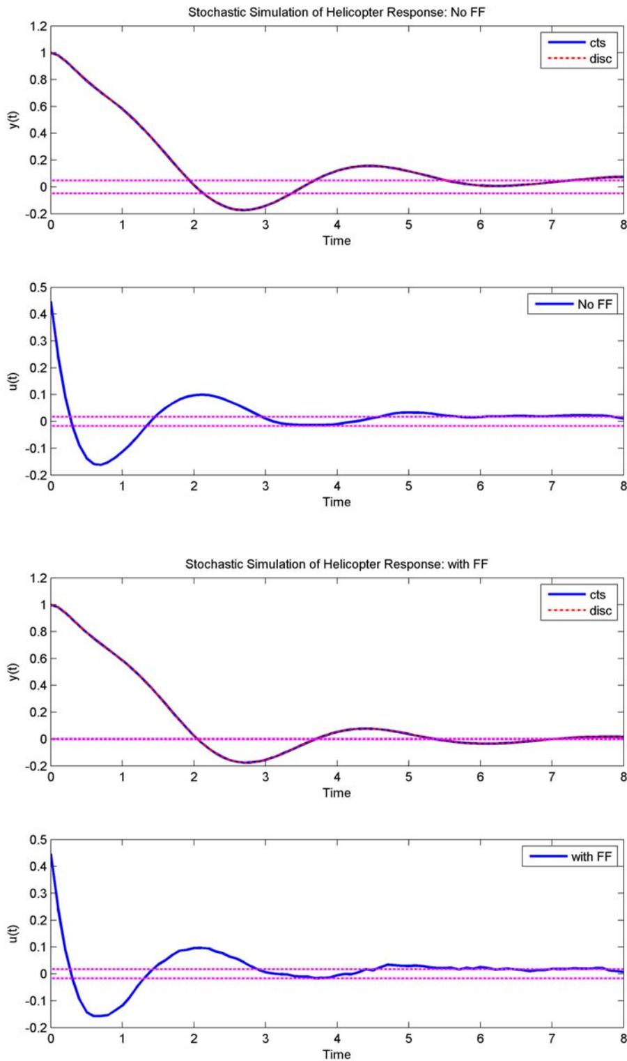
Figure 12.3: Stochastic Simulations with and without disturbance feedforward.
