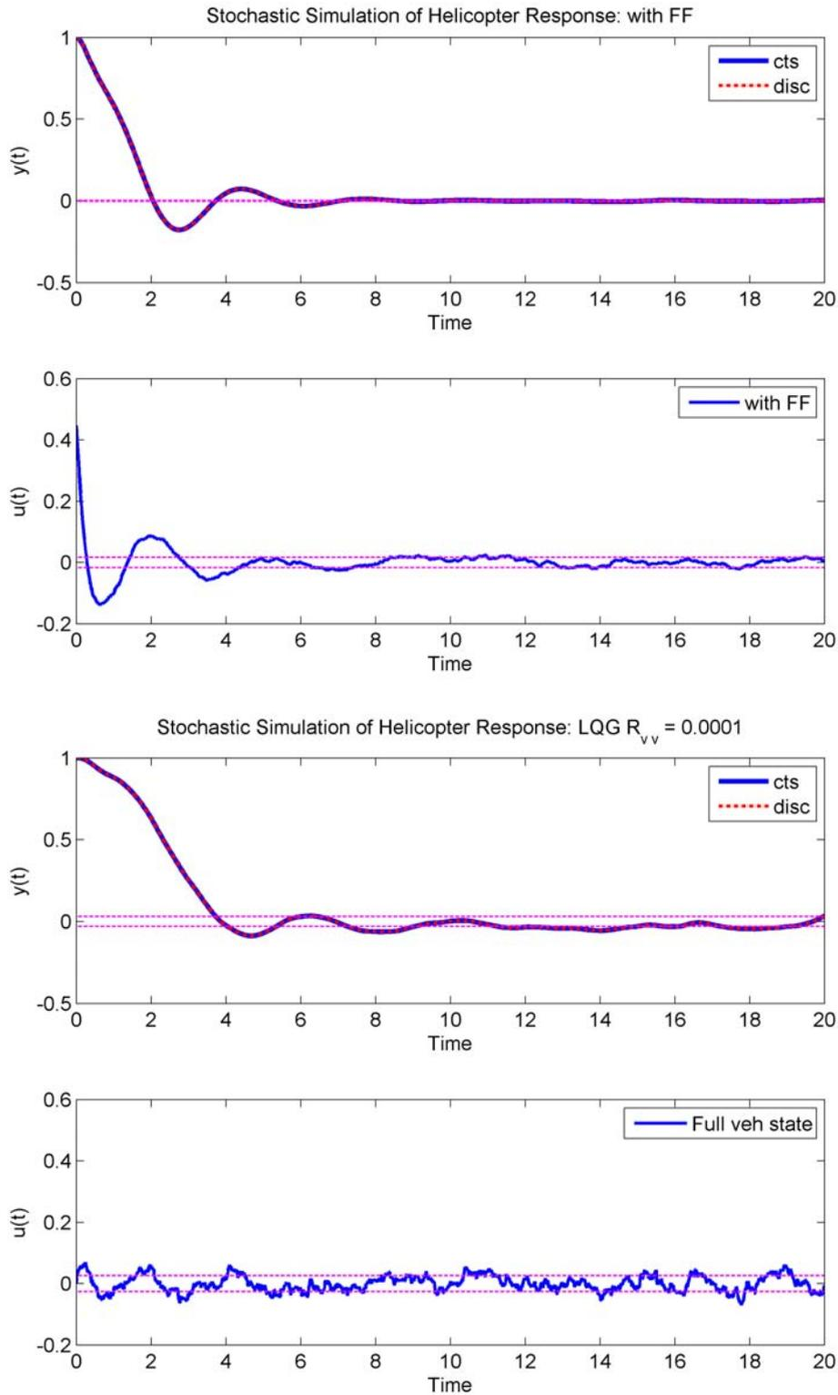
Figure 12.4: LQR with disturbance feedforward compared to LQG
