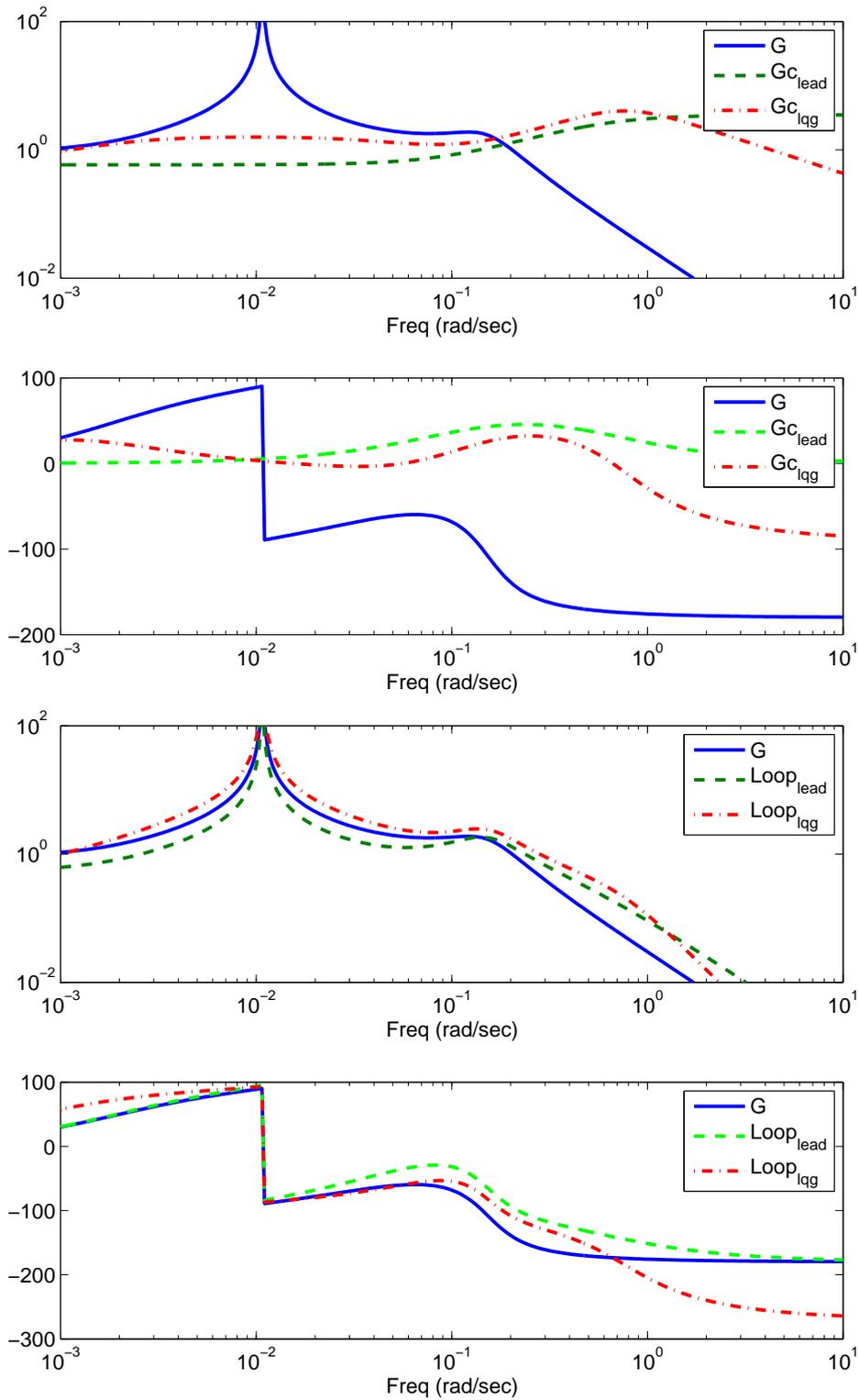
Figure 12.8: B747: Compensators and loop TF
