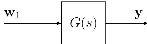
– New picture: system is  $y = G(s)w_2$ , with shaped noise input
