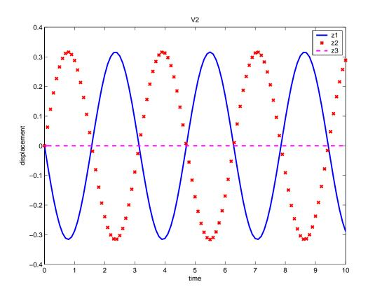
• Eigenvectors with that correspond with more constrained motion of the system are associated with higher frequency eigenvalues
