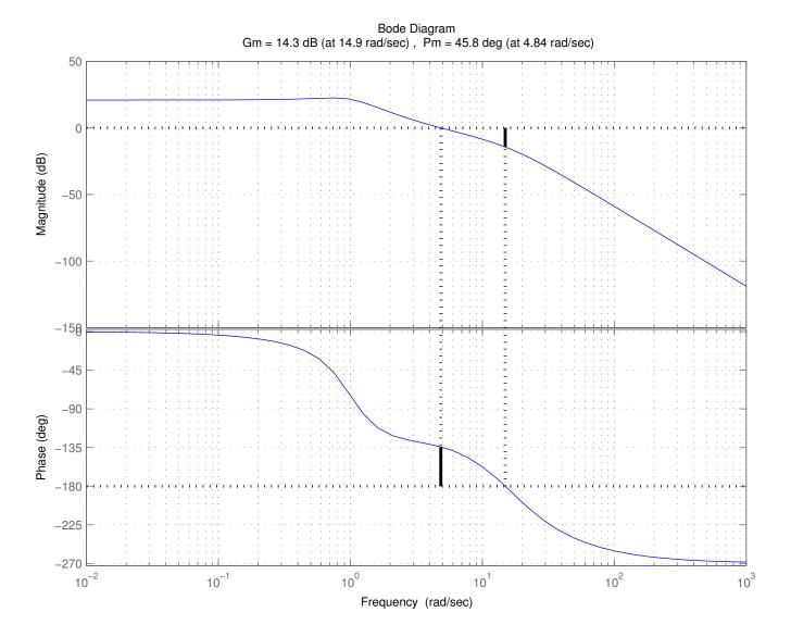
Figure 6: Quite significant gain and phase margins.
