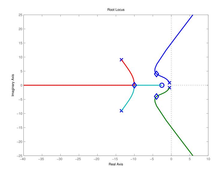
Figure 7: Freeze the compensator poles and zeros and draw a root locus versus an additional plant gain  $\alpha$ ,  $G(s) \Rightarrow \tilde{G}(s) = \frac{\alpha}{(s^2+s+1)}$ . Note location of the closed-loop poles!!
