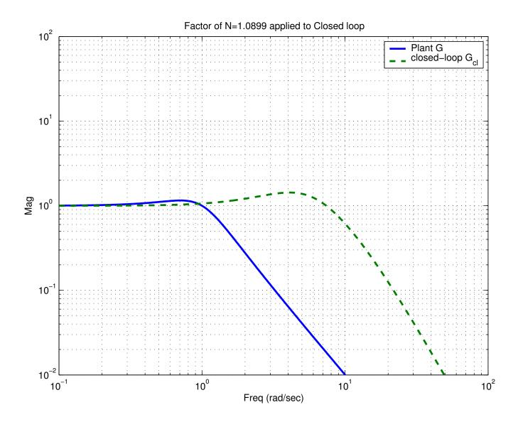
Figure 8: Closed-loop transfer - system bandwidth has increased substantially.
