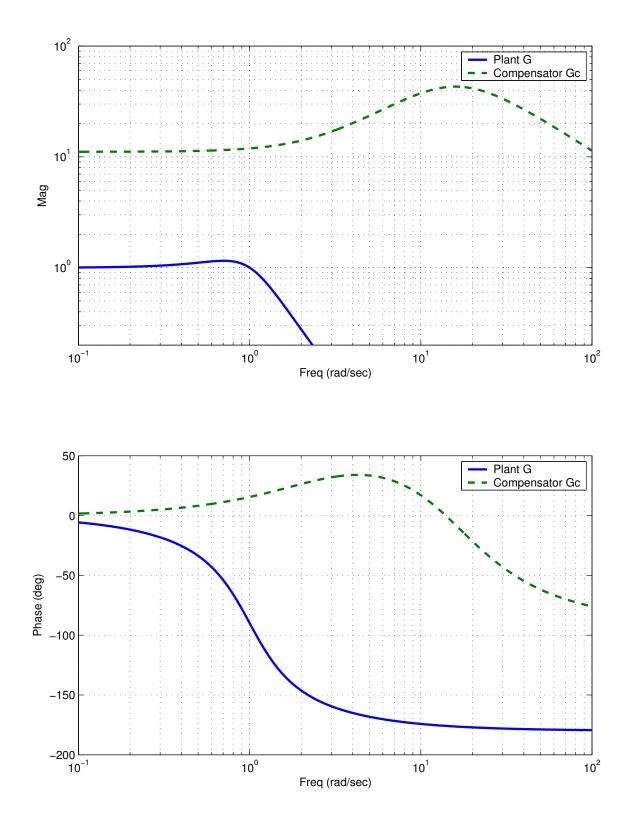
Figure 4: The compensator does indeed look like a high frequency lead (amplification from 2–16 rad/sec). Plant pretty simple looking.
