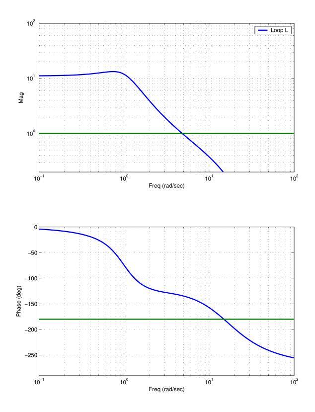
Figure 5: The loop transfer function  $L = G_c G$  shows a slope change around  $\omega_c = 5$  rad/sec due to the effect of the compensator. Significant gain and phase margins.
