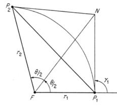
$$\sqrt{r_1r_2} = \begin{cases} FN\cos\frac{1}{2}(E_2-E_1) & \text{ellipse} \\ FN & \text{parabola} \\ FN\cosh\frac{1}{2}(H_2-H_1) & \text{hyperbola} \end{cases}$$
