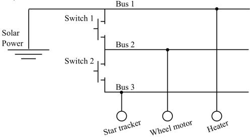
The star tracker, wheel motor, and heater each have a power indicator, which outputs 1 if the device is receiving power and 0 otherwise. Assume that these three devices and their indicators are working correctly; the solar panel is exposed to the sun, and the star tracker and heater are powered, but the wheel motor is **not** powered, as indicated on the figure below.
