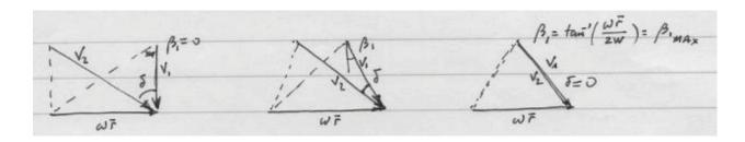
It is clear that as  $\beta_1$  increases (left to right),  $\delta$  decreases. So, the smallest  $\beta_1$  angles give the highest blade loading (most flow turning).
