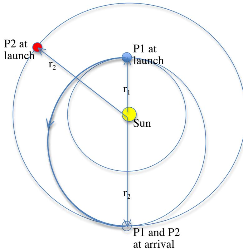
Assume that the planetary orbits are circular. Then it is clear that the trajectory of least energy which will allow the transfer is that which is just tangent to the orbits of the home and target planets; this is called the Hohmann transfer orbit, which is the half-ellipse that is sketched in the figure. The Heliocentric velocity at the start of this Hohman arc is the periapsis (perihelion in this case) velocity, as described at the end of the last lecture:
