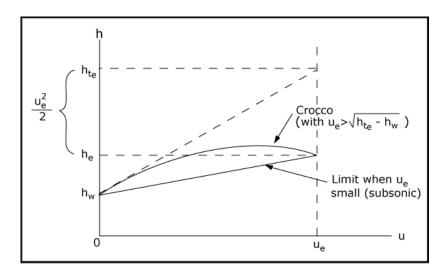
Note that whenever  $u_e > \sqrt{h_{t_e} - h_w}$  there develops an intermediate temperature maximum. But in any case, the wall slope is as if the line were coming from  $h_{t_e}$ , not from  $h_e$ . The case when  $h_e < h_w$  is more revealing even:
