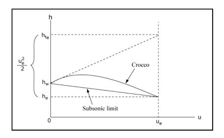
Now the wall slope is seen to be positive (heat into the wall), despite  $h_e < h_w\,$  (as long as  $h_{t_a} > h_w\,)$
