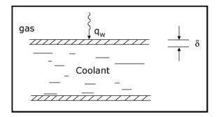
One would have  $q_w = K \frac{\Delta T}{\delta}$  where  $\Delta T$  is the temperature drop through the metal . As an initial guess, suppose the metal were stainless steel (K = 20 W / m / K), and  $\delta = 1$ mm. Then
