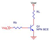
**Reminder** of something we covered in lecture too quickly: the voltage drop across a transistor (between the base and the emitter) is 0.6V in general, like in a diode.
