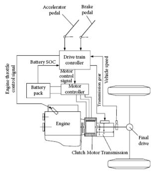
The electric motor is added in parallel to the engine. In the transmission, the torque converter is eliminated, leading to better efficiencies at low speeds. The engine is also turned off at low speeds and during idling...the electric motor is used to restart the engine or to drive the vehicle at very low speeds.
