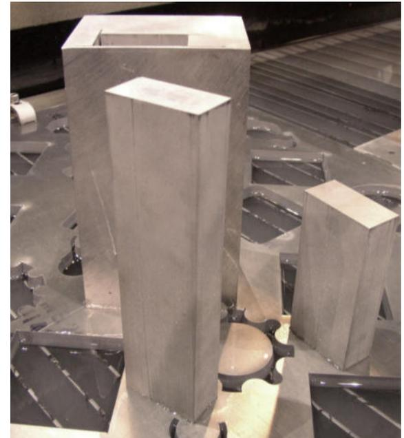
*This piece was made from 8" (200mm) thick aluminum as a demonstration of what an abrasivejet can do*
