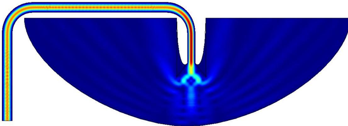
Figure 2. Power flux output plot. Dark blue corresponds to  $130\text{W/m}^2$ .  $127\text{W/m}^2$  is required to furnish  $400\text{W}$  to a  $2\text{m}$  diameter rectenna.
