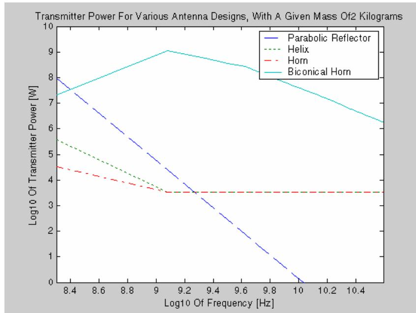
**Figure ?**. Relation Between Transmitter Power And Frequency (For A Given Mass)
