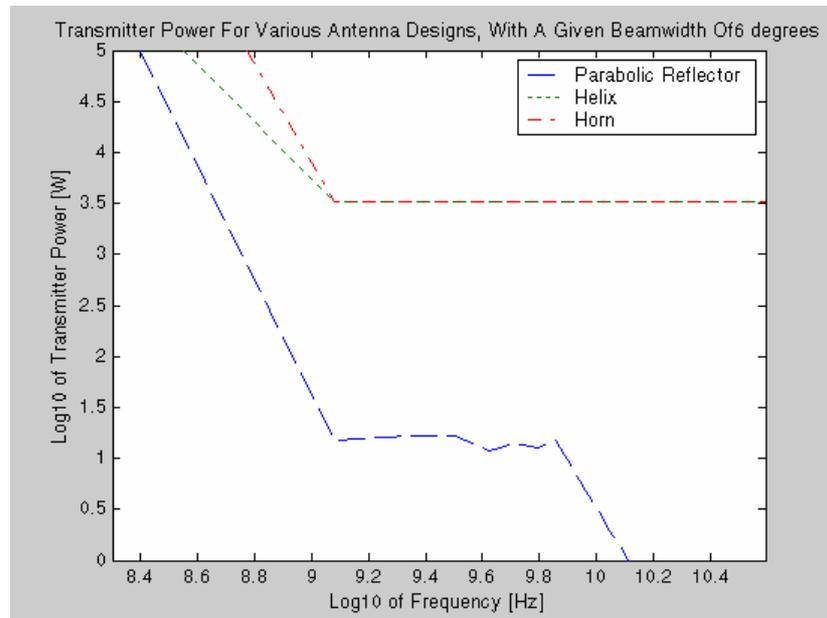
**Figure ?.** Relation Between Transmitter Power And Frequency (For A Given Beamwidth)
