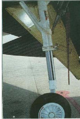
Figure 32. Outrigger gear located at the wingtips [29]
