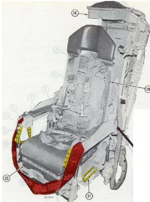
Figure 48. Upward ejection seat from the B-52 [27]
