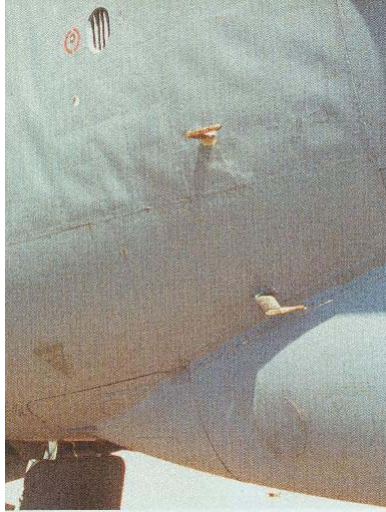
Figure 53. Two pitot tubes located on the starboard side of the B-52 [29]
