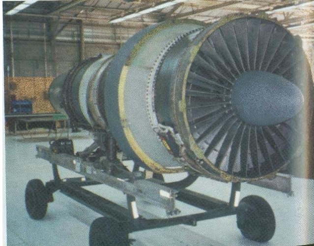
Figure 23. Pratt and Whitney TF33 turbofan used on the B-52H [29]
