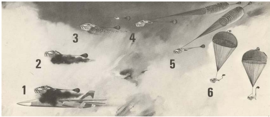
Figure 53: Ejection Sequence [F-111 Escape Module, Phillips]
