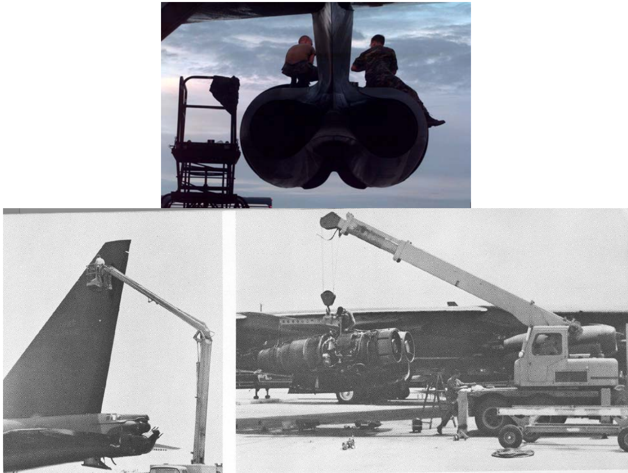
Figure 61. Engine maintenance on the TF-33 engines (above). The behemoth size of the B-52 requires the use of cranes, bucket trucks and other heavy machinery. [25] [26]
