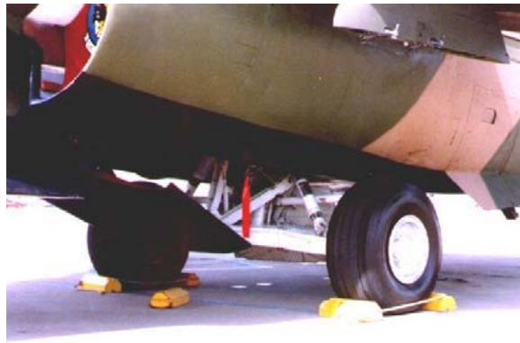
Figure 48: F-111 Main Landing Gear [18]
