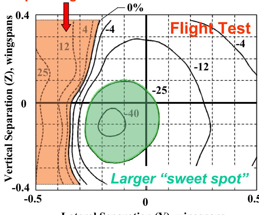
Calculated induced drag change obtained from **flight data**, with similar results at ALL flight conditions!
