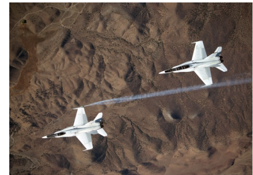
NASA Dryden Flight Research Center Photo Collection http://www.dfrc.nasa.gov/gallery/photo/index.html NASA Photo: EC01-0328-12 Date: November 9, 2001 Photo by: Carla Thomas Smoke generators show the helical paths of wingtip vortices behind two NASA Dryden F/A-19s used in the Autonomous Formation Flight (AFF) program during flight #743.
