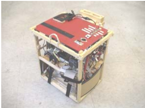
OHS Avionics Box
