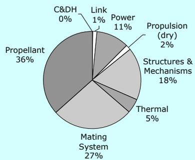
**Figure 10-9 Mass breakdown of Electric Cruiser design**
