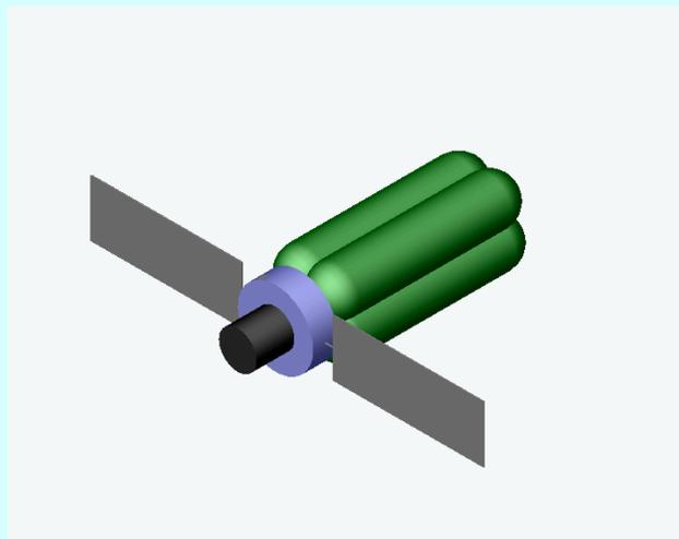
**Figure 10-6 Cryo one-way tug, showing extremely large fuel tanks; Bi-prop tug appears similar**
