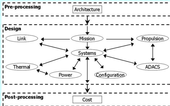
Figure 10-3 Spacetug ICE model components and interactions
