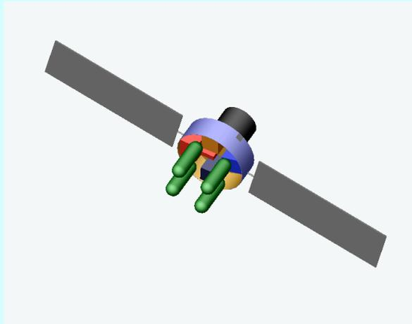
**Figure 10-7 Electric Cruiser (GEO round-trip tug)**
